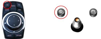
In the vehicle's **CD/Multimedia** menu, activate **AUX front** by iDrive and after it **long press CD-button** respectively **long press Menu-button** to choose the v.LOGiC as current AVsource.
