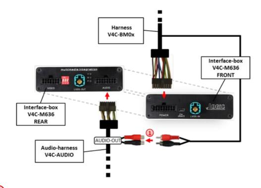
Connect the audio-RCA of harness V4C-BM0x to the female RCA-connectors AUDIO OUT of the audio-harness V4C-AUDIO.
