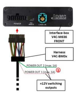
(1) You can configure the both +12V trigger outputs separately. The pink wire is POWER OUT 1 and the green wire is POWER OUT 2.
