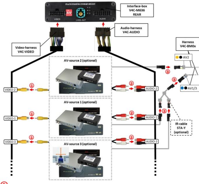
(1) Connect video RCA of AV-source 1 to female RCA connector VIDEO-1, the video RCA of AV-source 2 to female RCA connector VIDEO-2 and video RCA of AV-source 3 to female RCA connector VIDEO-3 of the video-harness V4C-VIDEO.
