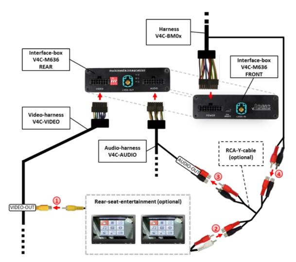
(1) Connect the video RCA of the rear-seat-entertainment to the female RCA connector VIDEO-OUT of video-harness V4C-VIDEO.
