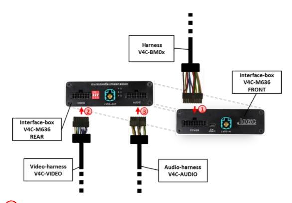
Connect female 18pin Micro-Fit connector of harness V4C-BM0x to the male 18pin Micro-Fit connector (POWER) on the front of the interface-box V4C-M636.
