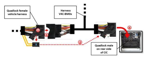
(1) Remove the female Quadlock connector of the vehicle harness from the rear of the navigation computer.
