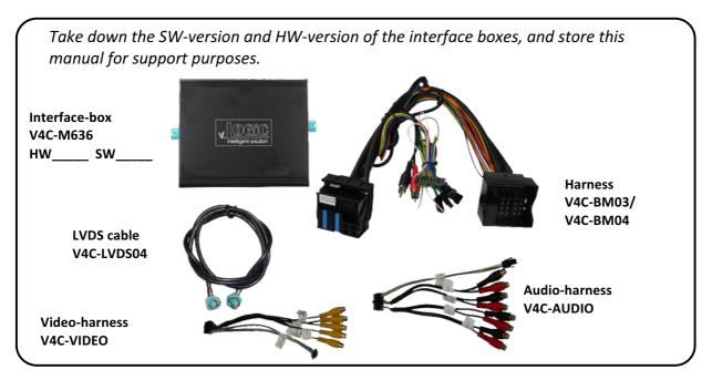
The V4-CIC-E package for BMW E-models contains harness V4C-BM03. The V4-CIC-F package for BMW F-models contains harness V4C-BM04. The harness will be referred to as V4C-BM0x in this manual.
