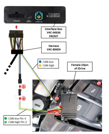
(1) Remove the iDrive from the centre console and unplug the existing flat female 10pin or 4pin cable connector.
