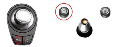
In **BMW** in the vehicle's **Entertainment** menu activate **AUX** and in **Mini** in the vehicle's **CD/Multimedia** menu, activate **AUX** front by iDrive and after it **long press MENU** button (1- and 2-button iDrive + Mini) to choose the interface as current AV-source.
