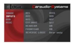
Note: The IR-control channel AV1 is preset to IR-Code 41 compatible DVB-T tuners
