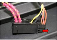
Loosen Pin 1 (yellow / white cable, CAN HIGH) and Pin 11 (yellow cable, CAN LOW) from the 20-pin socket and, as shown in the right-hand-side illustration, pin it in the included 3-pin socket.
