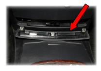
Remove the panel under the drawer (panel is slotted).
