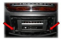
Open the drawer. Loosen the 4 Comand torx screws (2 respectively on each side).
