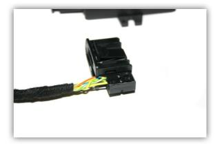
Insert completed connector into the plug on the backside of the navigation monitor. Connect 8pin Molex connector of TV-BM65 to CAN-box TV-401.
