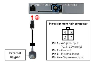
Connect the female 4pin connector of the keypad to the male 4pin connector of the video-interface.
