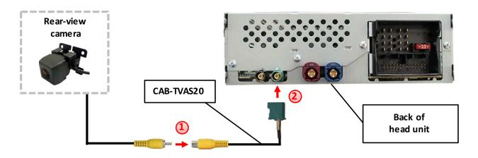
Connect the video RCA of the after-market rear-view camera to the female RCA connector of the CAB-TVAS20 cable.
