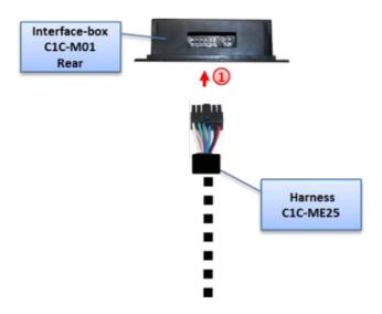
1 Plug harness C1C-ME25 into 12pin Molex of Interface-box C1C-M01.
